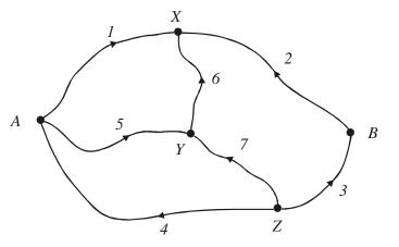
The weight of each observed height difference is inversely proportional to the distance in kilometres and the adjustment model is:  $P + \Delta H_{PQ} + v_{PQ} = Q$  where *P* and *Q* are the heights of points,  $\Delta H$  is the height difference and *v* is the measurement residual. All points are considered to be "floating"; hence there will be a datum deficiency and no solution by the usual means.
